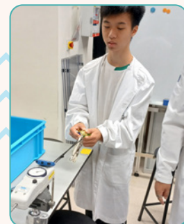
A student tests the tensile strength of a toy.
